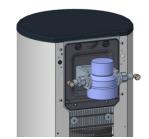
The filter cartridge must be replaced according to its filtration capacity and the water flow. At the latest, it must be replaced after 12 months following its commissioning or an interruption of more than 4 weeks.
